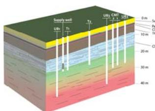
Fig. 3. Boreholes, red color indicates increasing salinity with depth
