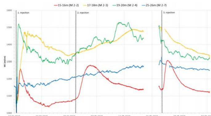
Fig. 6. Continuously registration of specific electrical conductivity (SEC) in 12 (four shown) monitoring filters between 14 – 26 m b.g.l. Vertical dotted lines indicate the times for tracer injection
