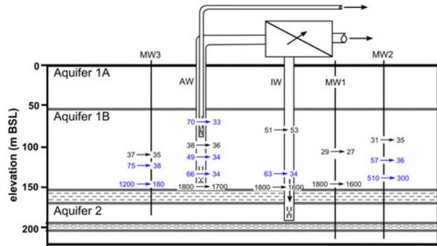
SEAWAT modelling suggested that the brackish water abstraction rate can be lowered to  $16 \text{ m}^3/\text{h}$  to keep chloride concentrations in the abstracted freshwater well constant at  $45 \text{ mg/L}$ .
