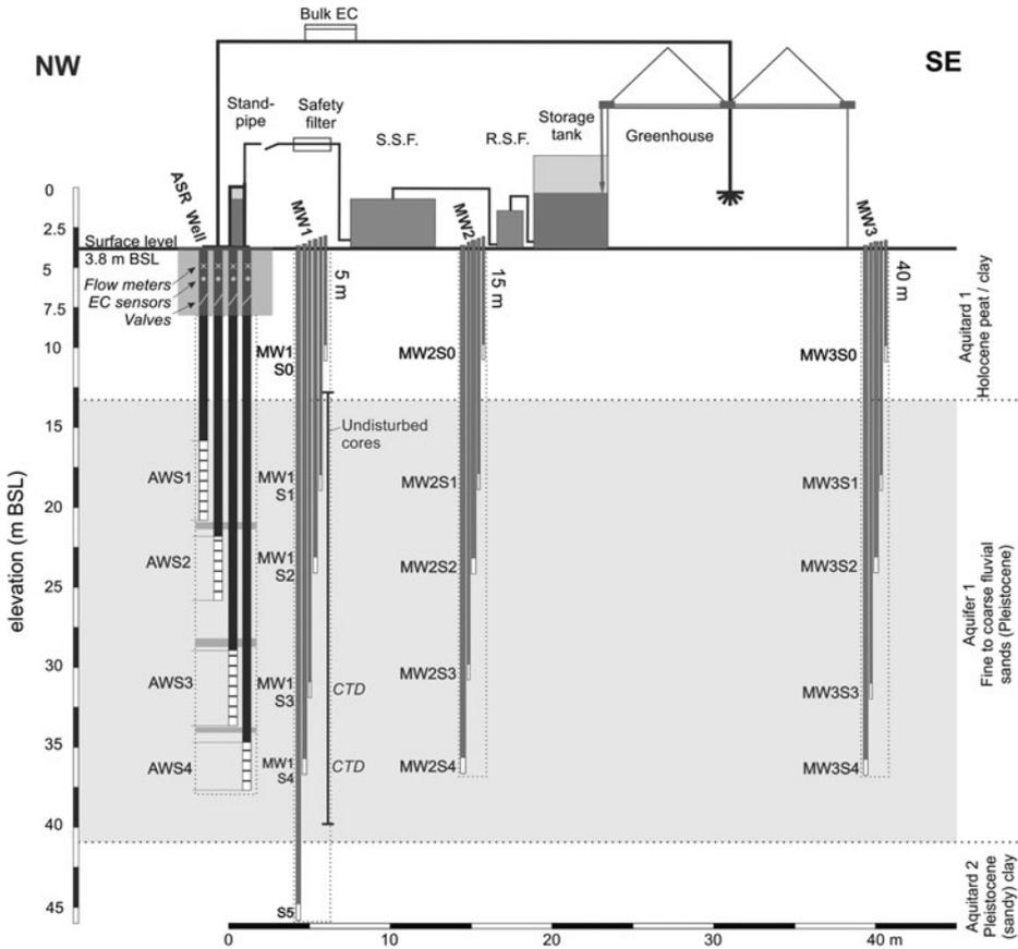
**Fig. 4** Cross-section of the Nootdorp ASR system as presented in Zuurbier et al. (2014). Water from the greenhouse is first pre-treated by rapid sand filtration (R.S.F.) and slow sand filtration (S.S.F) and then injected mainly by deeper wells in the aquifer, whereas recovery occurs from the shallow wells
