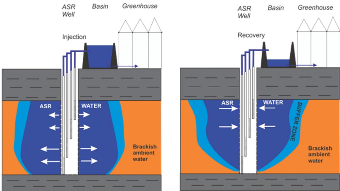
Figure 2-3 Cross-section of the ASR-Coastal set-up and operation: use of an MPPW in a single borehole that injects freshwater mainly in deeper parts of the aquifer and recovers water in shallower parts. This overcomes the early recovery of brackish or saline ambient groundwater at the bottom of the aquifer due to buoyancy forces.
